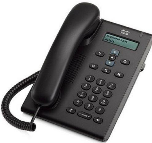
The Cisco Unified SIP Phone 3905 provides voice communication over an Internet Protocol (IP) network. The Cisco Unified IP Phone functions much like a digital business phone, allowing you to place and receive phone calls. In addition, the Cisco Unified SIP Phone 3905 supports features such as mute, hold, transfer, conference, call forward, and more.
